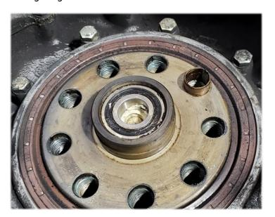
The old Pilot Bearing came out slick as a whistle. The newly compacted white bread plug was then removed with a screw driver revealing a clean space devoid of bread. So, I guess those crafty German engineers knew what they were talking about when they recommended using bread to remove a Pilot Bearing. White Bread!
