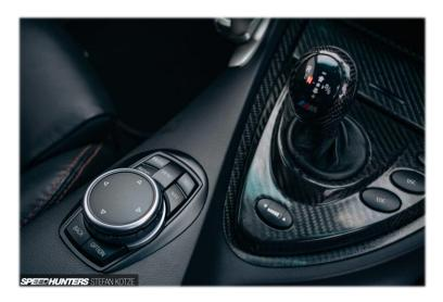
Wessel also installed the much newer NBT version of BMW's iDrive system, with performance gauges, navigation and automatic climate control.
