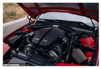
Although the donor engine was in good condition, Wessel wanted to ensure there'd be no trouble down the line as S85s are known to run bearings, even at relatively low mileage. The motor was completely rebuilt with forged pistons, forged con-rods, and race bearings. A full exhaust was also built for the
